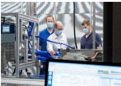
Expertise: MAHLE engineers working on a fuel cell with cooling system at the Stuttgart H2 test center
