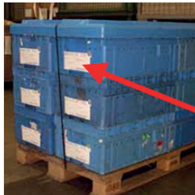
Fig. 18: Labeling pallet with small load carriers
