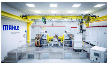
Focus on e-mobility: MAHLE test rig for electric drive axles at Fellbach near Stuttgart.
