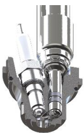
The MAHLE Jet Ignition makes hydrogen combustion in Liebherr motors possible.
