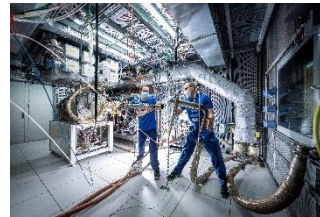
Many MAHLE core competences like thermal management are highly relevant for fuel cell applications. In this picture, MAHLE employees are testing cooling systems for fuel cell applications.
