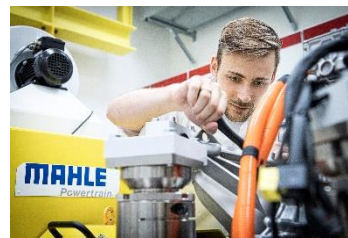
Mounted between two load machines, the e-drive is tested under real driving conditions.
