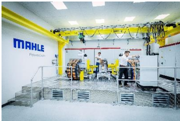
MAHLE Powertrain's test bench facilitates the accurate testing of electric drives, ensuring that electric vehicles are safe and reliable.
